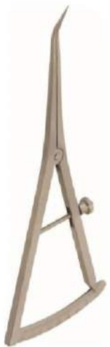
SI-1449 Measuring Loop angled length 175 mm measuring range 0-40 mm
